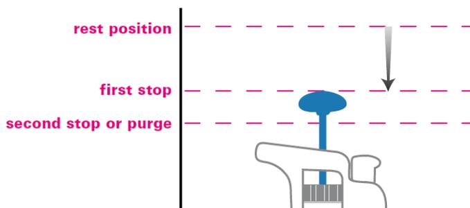
2. Holding the top vertical with the button held at the first stop, dip the tip into the solution. **Slowly** release the operating button, drawing the liquid into the tip. Withdraw the tip from the liquid without touching the sides of the vessel. **Never** turn the pipette
