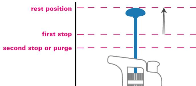
3. Dispense the liquid into the receiving vessel by **gently** pressing the operating button to the first stop, wait a half second, then press the button to the second stop. Remove the tip from the vessel, sliding it along the wall of the vessel. There should be no remaining liquid in the tip, and the operating button should be back in operating position
